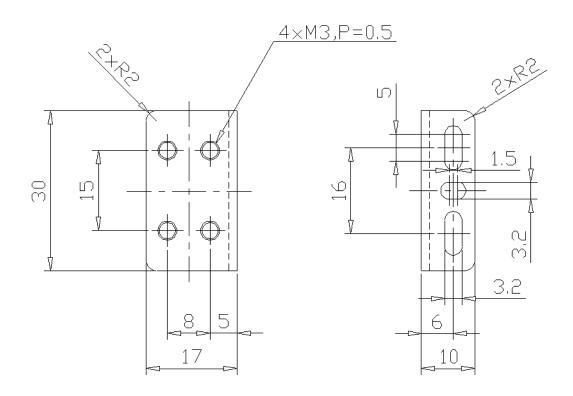
Material : SUS316L Supplied Accessories : Screw x2(M3,6mm,Stainless steel)
