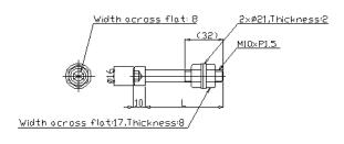
Nickel ploted steel L=45nm: DP-87406 L=65mm: DP-87407
