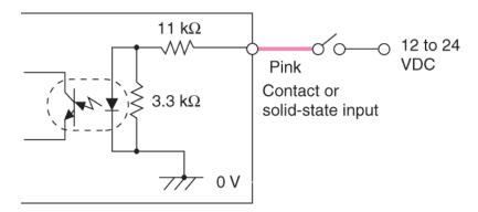
When the external calibration input is not used, cut the pink cable at the root, or connect this cable to the positive terminal of the power supply.
