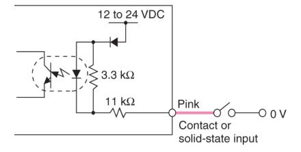
When the external calibration input is not used, cut the pink cable at the root, or connect this cable to the positive terminal of the power supply.
