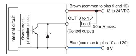
\* When OUT 15 is switched to STB, an over-current protection circuit is not provided.
