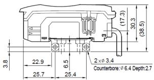
Bottom surface of amplifier mounting bracket
