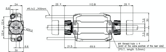
\* This space is needed for installing the fixing rings.
