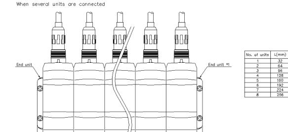
\*1 End units must be used when an expansion unit is connected. (Option)
