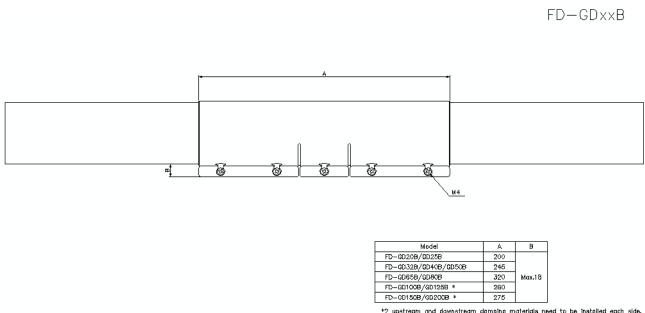
$^{*2}$  upstream and downstream damping materials need to be installed each side. Material: SUS304
