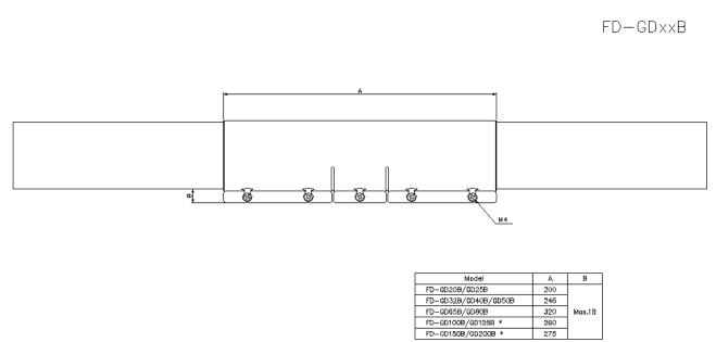
\*2 upstream and downstream damping materials need to be installed each side.
