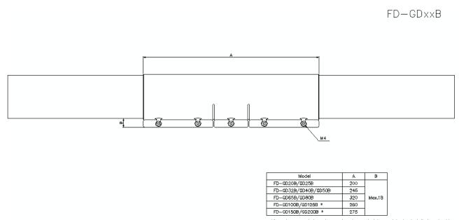
\*2 upstream and downstream damping materials need to be installed each side. Material:  ${\tt SUS304}$   ${\tt t=1.3}$
