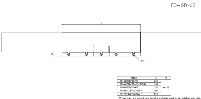
\*2 upstream and downstream damping materials need to be installed each side.  ${\tt Material:SUS304}$
