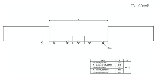
\*2 upstream and downstream damping materials need to be installed each side.  ${\tt Material:SUS304}$
