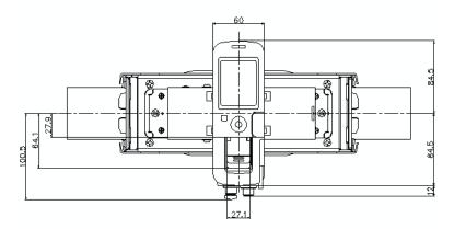
When power supply and Ethernet cable are connected
