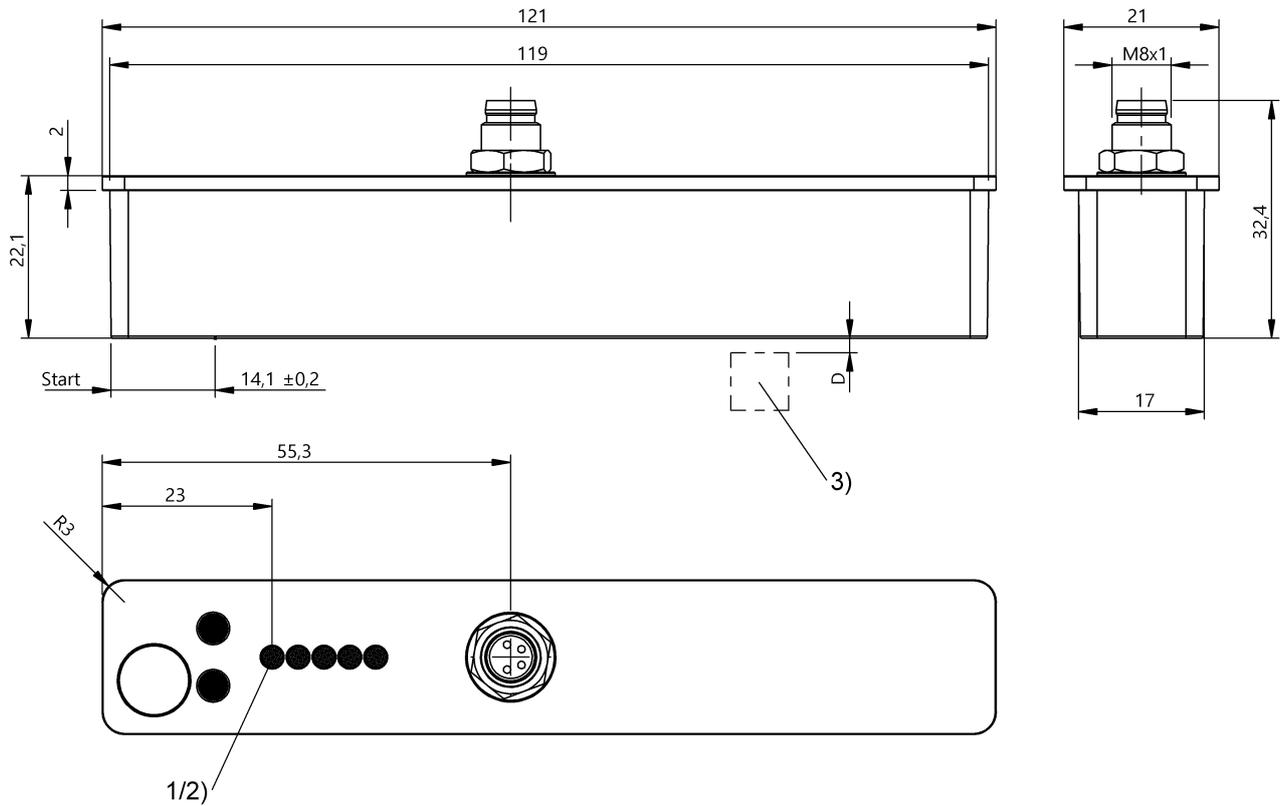
1) LED Power, 2) LED function indicator, 3) Encoder
