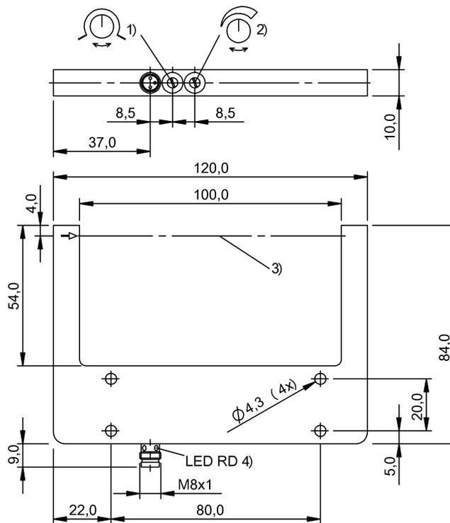
1) Light-on/dark-on, 2) Sensitivity, 3) Optical axis, 4) Output function
