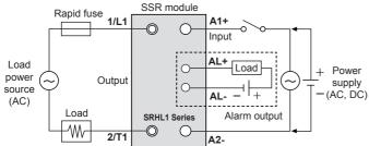
%Alarm output terminals (TTT) are only for the rated load current 40A model (SRHL1-\_\_40\_).
