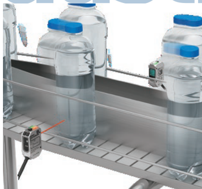
Presence detection of plastic bottles
